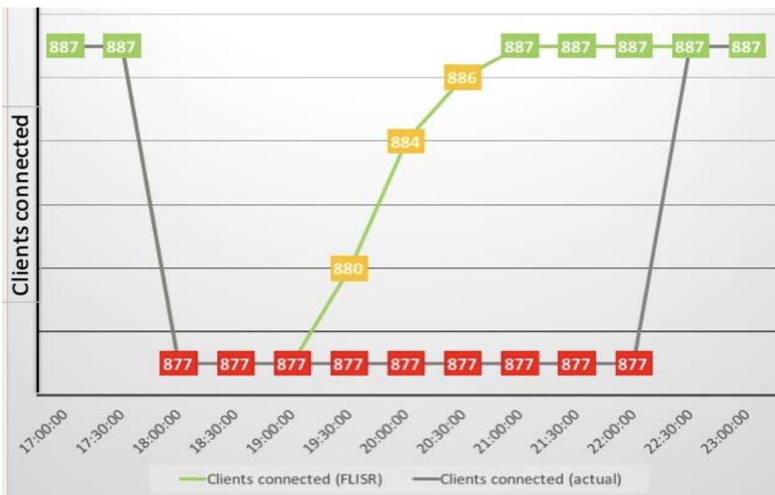
Figure 2: Timeline of a single interruption in the LV grid controlled by CEZ Romania - Status Quo (without) vs. with FLISR utilisation
